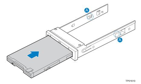
Figure 25. Inserting a Drive into the Floppy Conversion Kit Carrier
